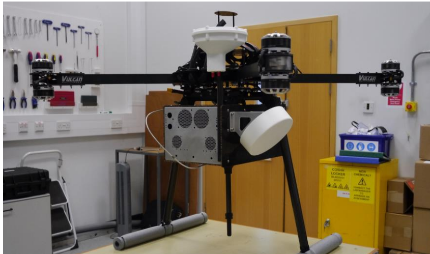
Figure 12: Sensor enclosure mounted on Raven X8 multi-rotor aircraft
